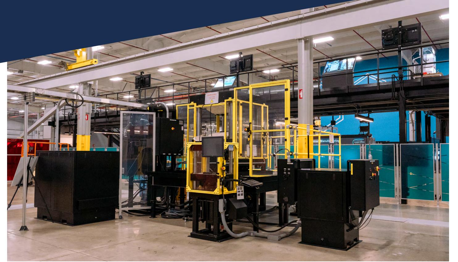
**Forming Presses** are often used for processing or reshaping material of various forms by thermomechanical deformation (a.k.a. upsetting). The workpiece and/or tool are often (but not always) held at elevated temperature, and pressure is applied by the press to deform the material into a predetermined geometry.
