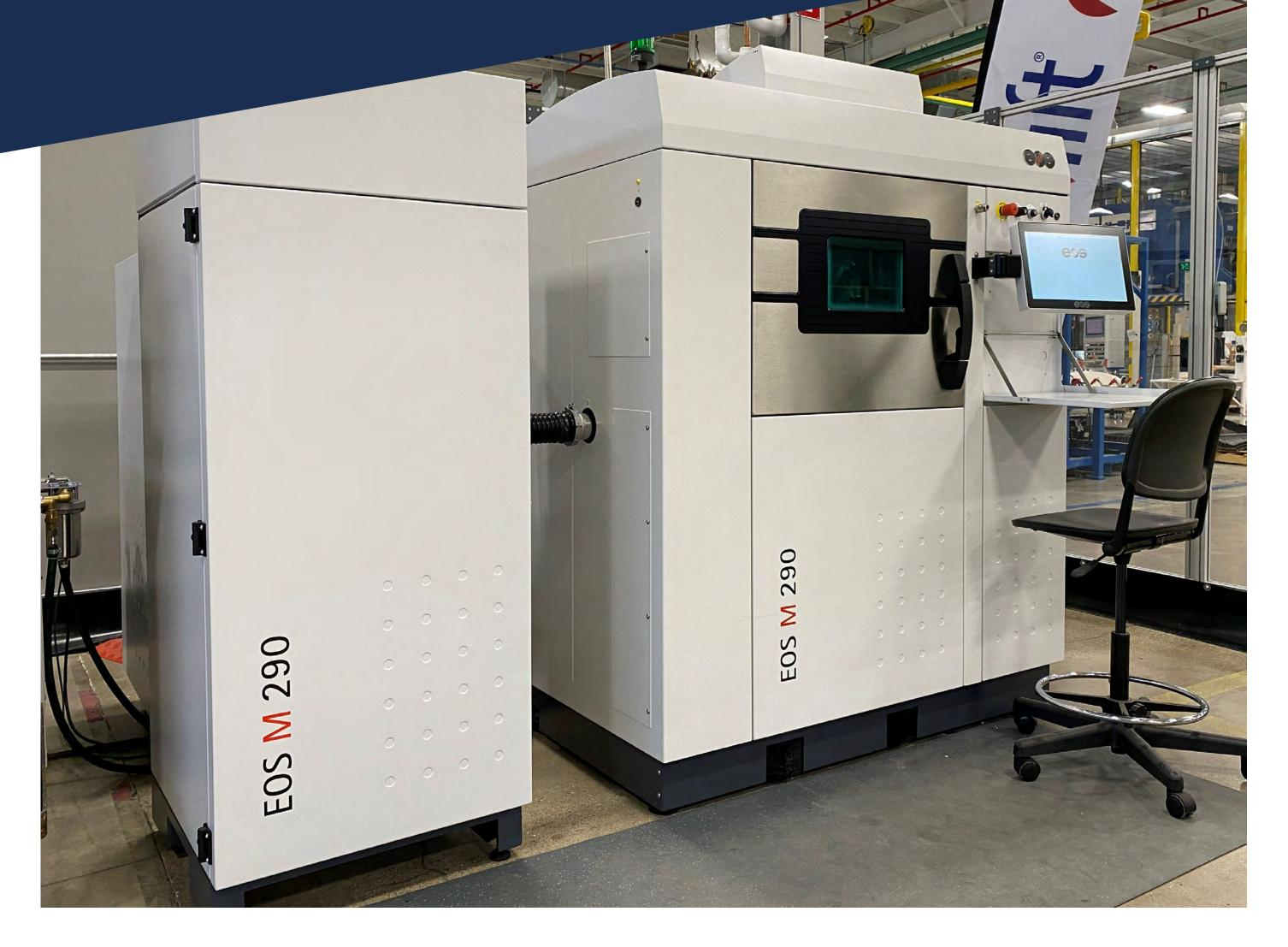
The award-winning EOS M 290 employs Direct Metal Laser Solidification (DMLS $^{\text{TM}}$ ) technology. This powder-bed based form of 3D printing ensures maximum part density and exceptional quality.
