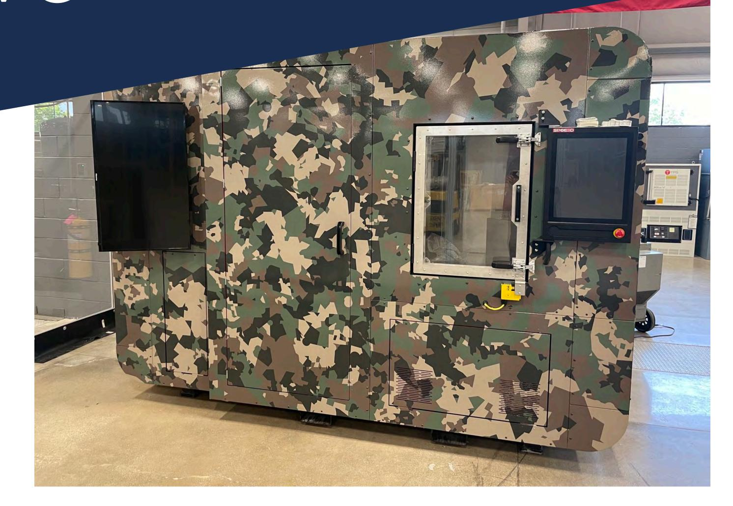
**Cold Spray Additive Manufacturing** employs low-temperature kinetic deposition of various types of metal powders, supporting the production of custom components and functionally-graded materials.
