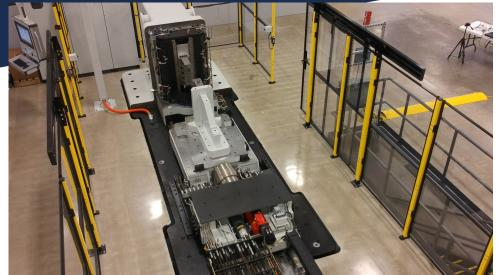
**Linear Friction Welding**, is a solid-state process in which one part moved in a linear motion at high speed and is pressed against another part held stationary. The resulting friction heats the parts, causing them to forge together.
