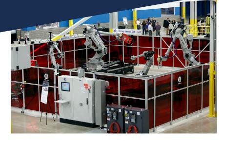
The **Flexible Joining System** can be used for many joining needs in the metalworking process, including wire-feed welding and spot welding, as well as fixturing, positioning, and alignment of components and assemblies.
